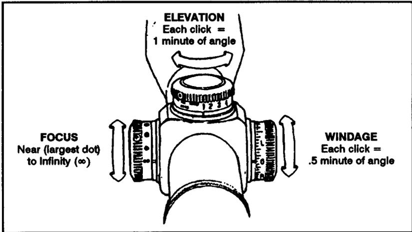
**Figure 2-18. Focus, elevation, and windage adjustment dials.**
