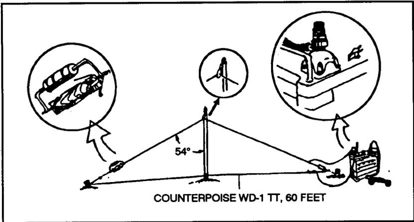
**Figure 7-9. Vertical half-rhombic antenna.**
