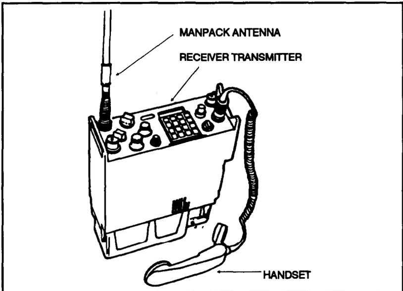
**Figure 2-36. AN/PRC-119 radio.**
