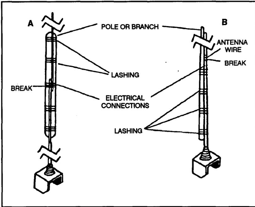
**Figure 7-1. Emergency repair of broken whip antenna.**
