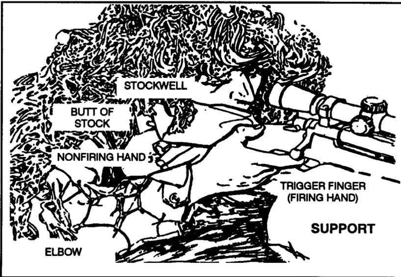
Figure 3-1. Firing position.
