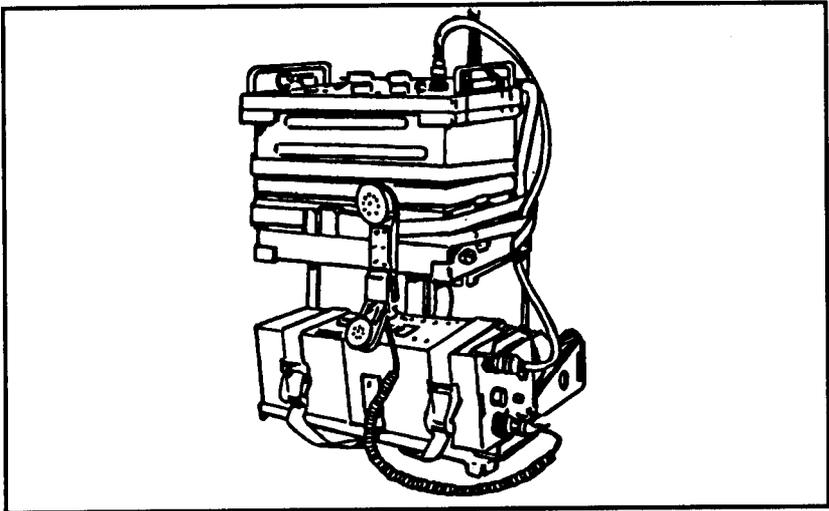
Figure 2-34. AN/PRC-77 radio.
