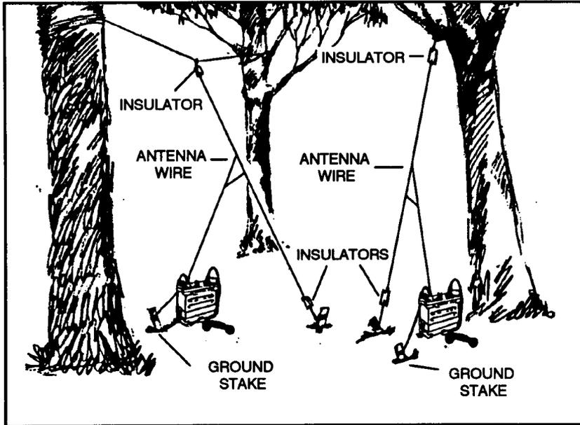
Figure 7-8. Improvised vertical half-wave antenna.
