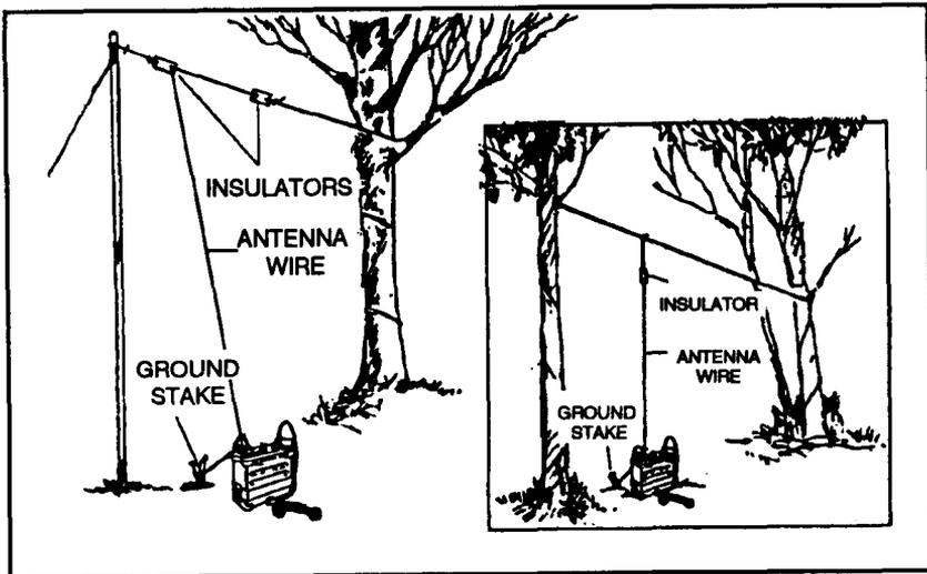
**Figure 7-4. Additional means of supporting vertical wire antennas.**
