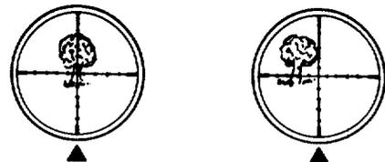
WHEN THE EYE IS CENTERED IN THE SCOPE AND THE CROSSHAIR APPEARS CENTERED ON THE OBJECT THEN YOU MOVE YOUR HEAD SLIGHTLY TO THE LEFT AND THE OBJECT MOVES OFF CENTER OF THE SCOPE PARALLAX IS PRESENT. NO PARALLAX IS PRESENT WHEN THE HEAD CAN BE MOVED SLIGHTLY IN ANY DIRECTION AND THE CROSSHAIR STAYS CENTERED ON THE OBJECT.
