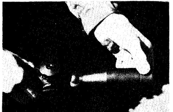
Figure 2-8. Final Stage of Focusing Objective Lens.
