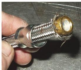
**Step Six:** Grab a suitable tapered punch and expand the teflon liner into the I.D. of the ferrule firmly.
